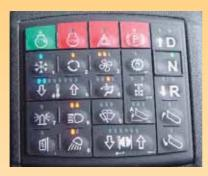
Both operator or site selectable maximum speed control allows the vehicle to automatically de-accelerate and apply the retarder to prevent onsite speeding.
