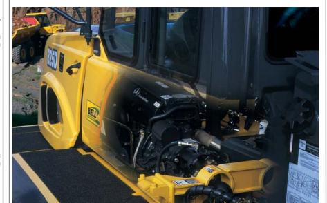
Semi-independent, quad rubber mounted leading arm linkages supperted by nitrogen and oil filled struts.
