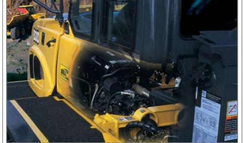
Semi-independent, quad rubber mounted leading arm linkages supported by nitrogen and oil filled struts.
