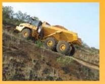
• The incorporation of a Pitch and Roll sensor in the vehicle allows the bin to not be operated if the truck is in an unsafe position.
