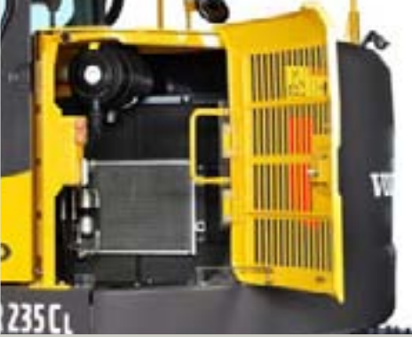
• Ground level air filter access.
