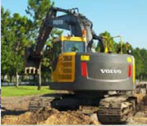
• Rounded design with a compact swing radius.
