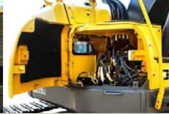
• Wide open, ground level service area provides easy hydraulic valve access.
