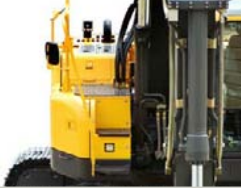
• 3-point, multi-purpose access with hand rail for ease and safety.
