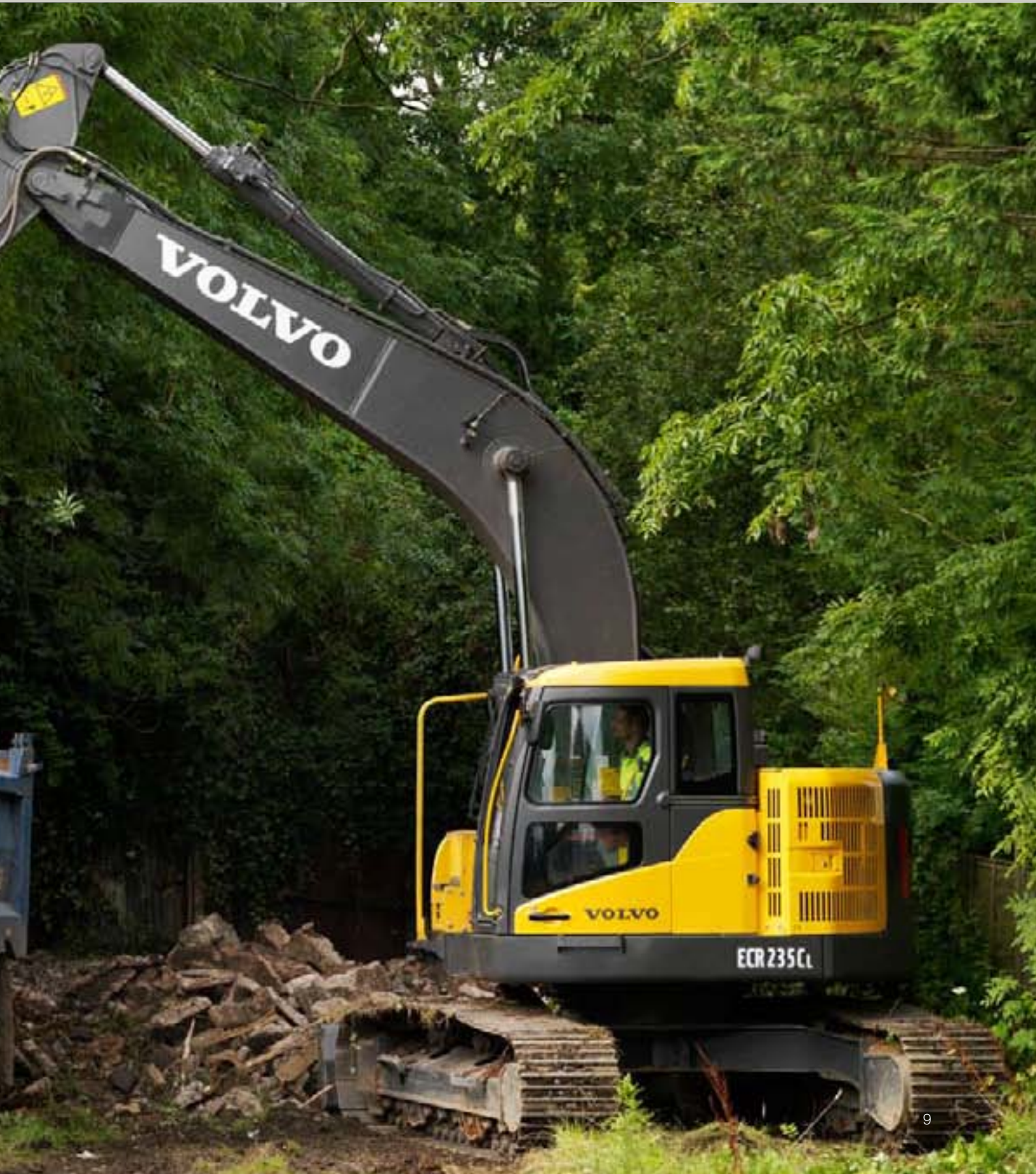
• 3-point, multi-purpose access with hand rail for ease and safety.
