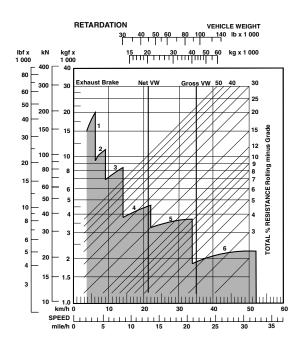
Instructions: From intersection of Vehicle Weight with Percentage resistance line read across to determine maximum Gear attainable, and then downwards for Speed.
