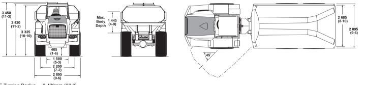
SAE Turning Radius Clearing Radius 8 470mm (27-9) 8 950mm (29-4)
