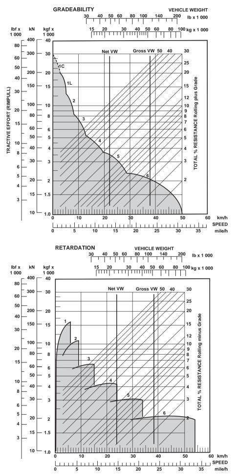
Instructions: From intersection of Vehicle Weight with Percentage Resistance line read across to determine maximum Gear attainable, and then downwards for Speed.
