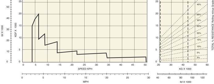
Instructions: From intersection of vehicle weight with percentage resistance line read across to determine maximum gear attainable, and then downwards for speed.
