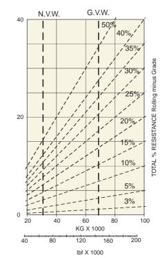
Instructions: From intersection of vehicle weight with percentage resistance line read across to determine maximum gear attainable, and then downwards for speed.
