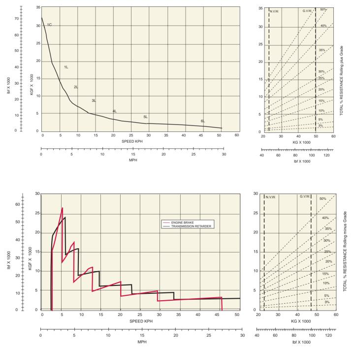
Instructions: From intersection of vehicle weight with percentage resistance line read across to determine maximum gear attainable, and then downwards for speed.
