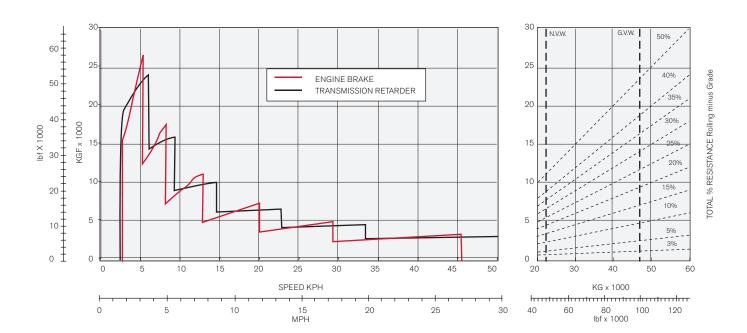
Instructions: From intersection of vehicle weight with percentage resistance line read across to determine maximum gear attainable, and then downwards for speed.
