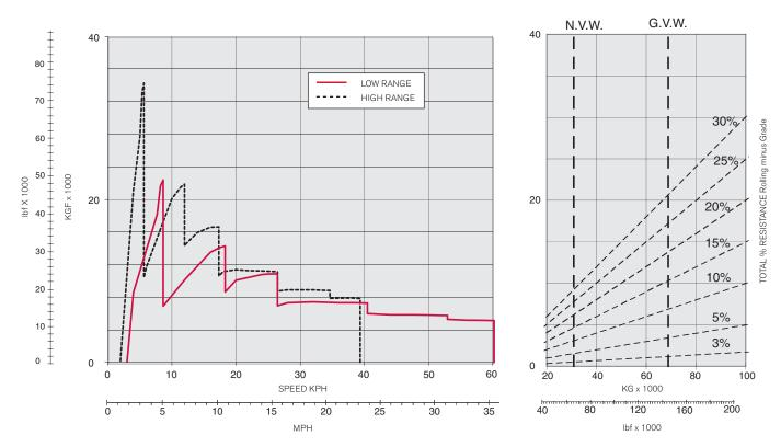
Instructions: From intersection of vehicle weight with percentage resistance line read across to determine maximum gear attainable, and then downwards for speed.
