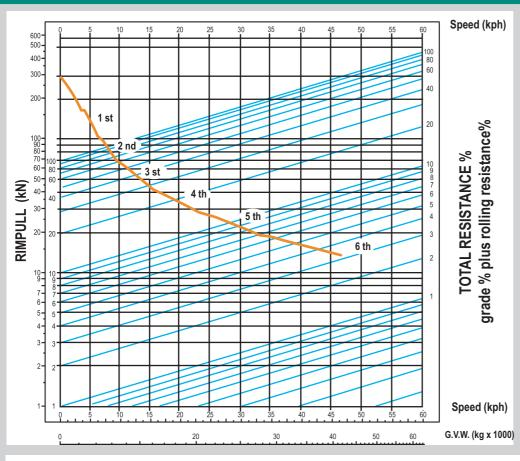
From the meeting between the M.T.T. of the vehicle and the inclined line corresponding to the total resistance %, to the left to determine the corresponding gear and, coming down,the max.speed of the vehicle.
