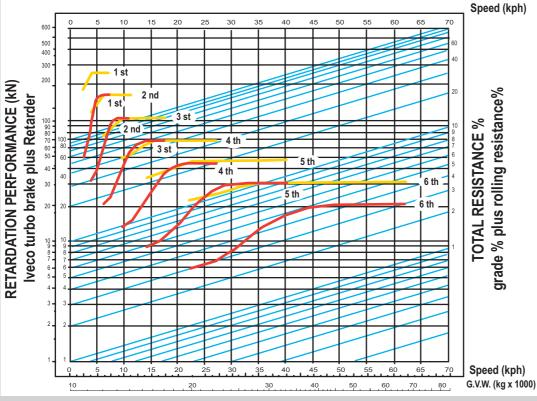
The curves in red refer to the motor's brake(STD); quelle in yellow, to the motor's brake plus retarder (OPT).
