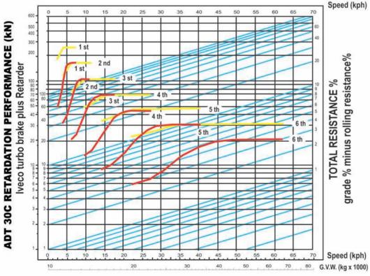
From the intersection of the vertical GVM line and the selected inclined rolling resistance line, draw a horizontal line to the left until the point where it runs under the first curve above it. Drop a vertical line from that point down to the speed scale and read off the maximum vehicle speed. The red curves depict engine brake retardation and the yellow curves depict the combination of engine brake and transmission retarder (where fitted) performance.
