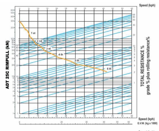
From the intersection of the vertical GVM line and the selected inclined rolling resistance line, draw a horizontal line to the left until it intersects the rim pull curve. Drop a vertical line from that point down to the speed scale and read off the maximum vehicle speed.
