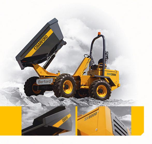
Conveyor belt shot blasting of components, primer and polyurethane oven bake paint system gives Barford dumpers a paint finish with life long durability and resilience to the elements
