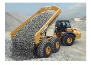
The Multiplex system allows the monitoring of all sensors and on-board diagnostics enable easy troubleshooting and access to all technical information. The computer controls the "smart management" of the body raising and lowering plus the integrated braking effect between the transmission retarder and engine brake for continuous, maximum performance.
