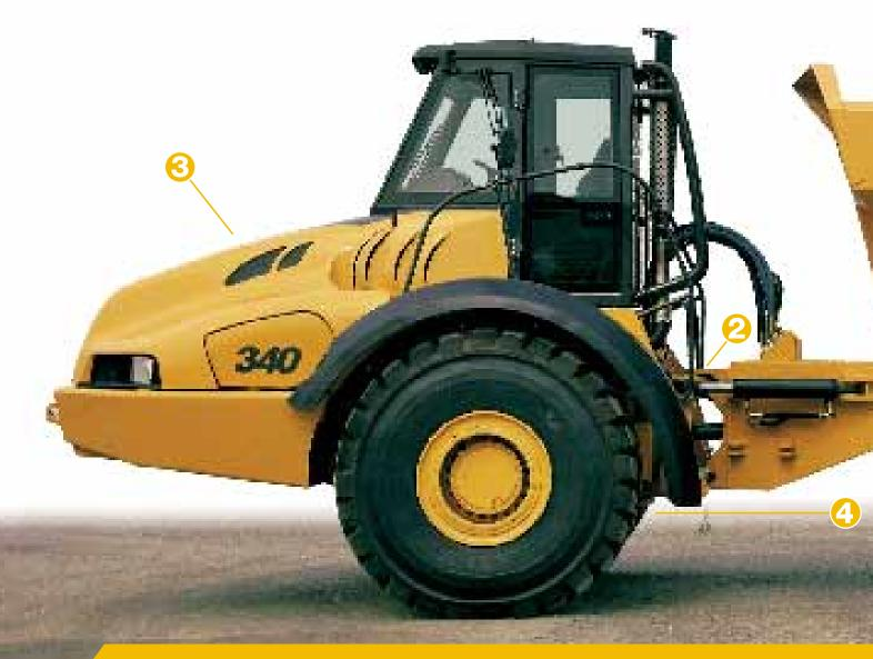
The widest **chassis** in the industry improves both traction and stability, in addition to allowing the use of inboard tipping cylinders. Not only does this location protect the cylinders from damage, the improved lift geometry allows for a much gentler initial tipping action, thus reducing long term component wear.
