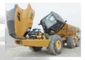
What could be simpler than stepping down from the cab and activating a switch opening the one-piece bonnet by its own electric-hydraulic mechanism? This design innovation makes daily or routine servicing much easier. By tilting the Cab up to 51 degrees and opening lateral mudguards, you obtain excellent access to the whole engine and transmission compartment and all main hydraulic components, simplifying all maintenance operations.
