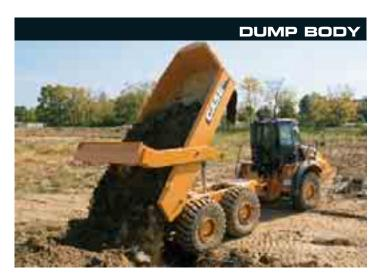
The Case B series articulated truck has a wide chassis and dump body to provide a lower centre of gravity, increasing stability on rough ground and assisting the suspensions system to provide a smooth ride. The tilt cylinders are mounted within the wide frame rails, for added protection and to improve the lift geometry for rapid discharge and return to hauling position.
