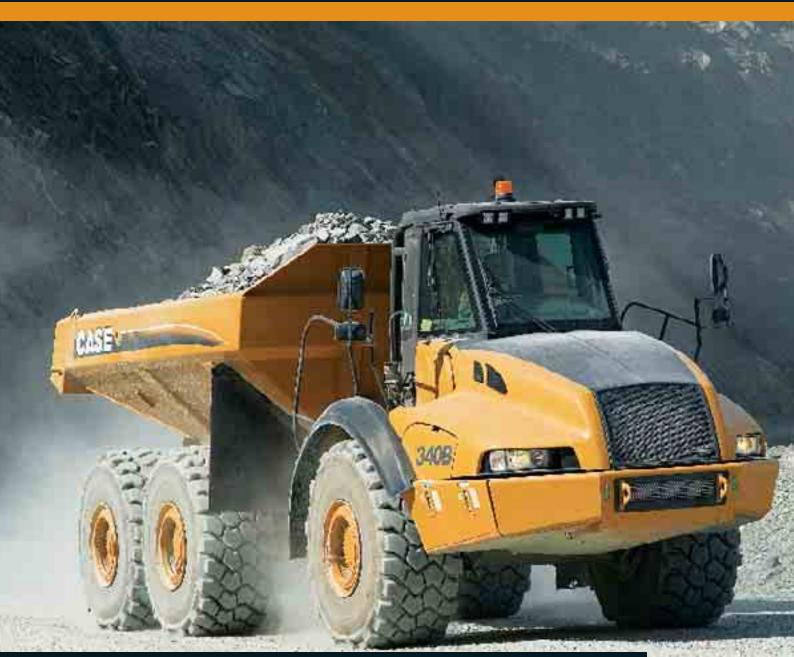
Engine Horsepower Payload Heaped capacity Total laden weight **327B** 235 kW/315 hp 24 650 kg 14.5 m<sup>3</sup> 46 890 kg **330B** 260 kW/349 hp 28 160 kg 17.6 m<sup>3</sup> 50 730 kg **335B** 306 kW/410 hp 31 500 kg 20.0 m³ 60 000 kg **340B** 340 kW/456 hp 36 000 kg 22.0 m<sup>3</sup> 65 000 kg
