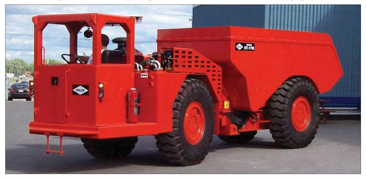
The DUX MODEL DT-17N, 15.4 tonne payload capacity high speed articulated haulage truck is only 1.98 meters wide and is well suited to operate in confined workings, small drifts and tunnel projects. The ruggedly built DT-17N is maintenance friendly guaranteeing long trouble free life with low operating cost-per-tonne on development projects and high capacity production hauling of ore, waste and backfill on level and ramps.
