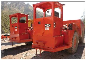
Optional bolted spacer raises FOPS/ROPS operator's compartment for excellent visibility in reverse driving. Sixteen DUX DT-17N's equipped with spacers are hauling excavated muck in a major water tunnel project in Chile.
