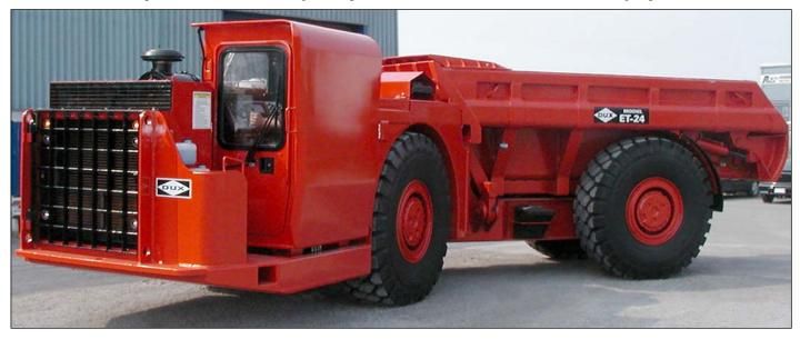
The DUX MODEL ET-24, 24 short ton (22 metric tonne) capacity compact profile articulated four-wheel drive ejector truck is designed for the transport of ore, waste rock and backfill on level and steep ramps in areas with extremely low headings.
