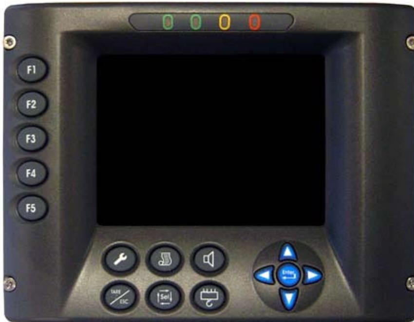
Before starting the lifting operation, the user must check that the operating mode set corresponds to the real machine's configuration ( boom, outriggers, counterweight, jib's length and angle, etc ) and the number of lines and confirming it pressing
