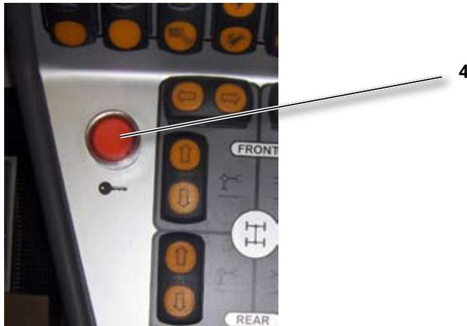
Release button **4** to re-enable limiter.
