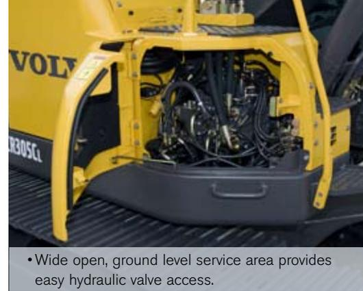
• Wide open, ground level service area provides easy hydraulic valve access.
