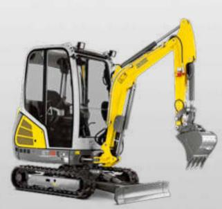
ET18 – the tiny powerpack Transport weight: 1,610 – 1,955 kg Equipment: Standard / telescopic undercarriage, VDS, Canopy / Cab Special characteristics: Most powerful machine in its class
