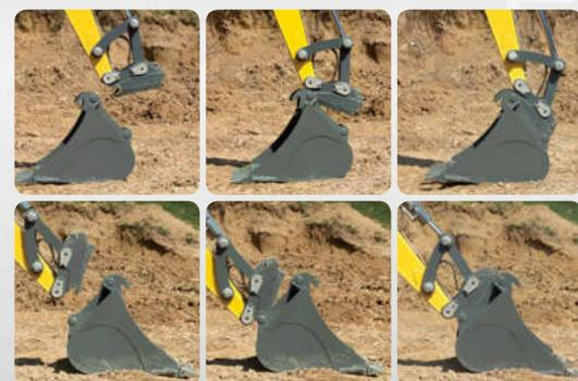
Smart deployment as backhoe and face shovel. By simply turning it around, the backhoe can be used as a face shovel. Not only does this save time, but it also increases the excavator's flexibility.
