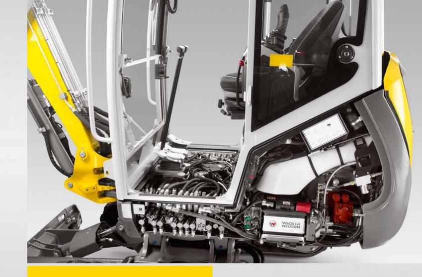
1 Cooler, longer-enduring and more robust. The ET-Series comes equipped with a unique cooling concept, guaranteeing extremely high thermal resistance thanks to a newly-developed cooling air circulation system. This lets you work under full load and at an ambient temperature of up to 45 °C. A generally lower temperature level in the hydraulic system as a whole ensures longer service life for components.
