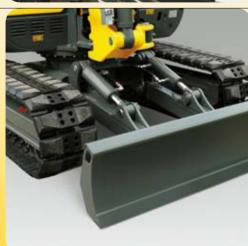
Durable hybrid tracks which can be driven easily over asphalt and sharp edged surfaces and whose links can be individually replaced.
