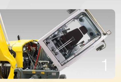
1 Generously dimensioned tipping cab with excellent all round view. A comfortable work place ... also an enormous safety factor. Unobstructed service access to all components.
