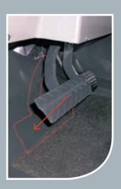
Keep 100% control when loading with one foot on the throttle and one foot on the inching pedal. The inching pedal slows forward movement without changing engine speed.
