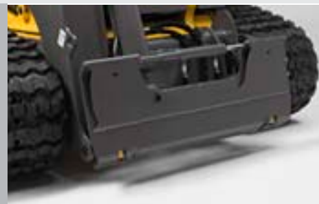
Volvo hydraulic attachment bracket allows the operator to change attachment from the seat (Included in the Deluxe package)
