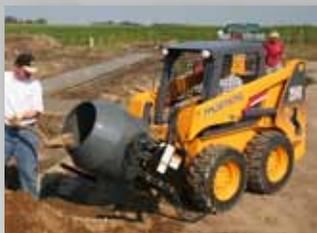
**STURDY ▲** Level II-certified ROPS/FOPS structure provides protection, yet allows an unobstructed view to the attachment and surrounding work area.
