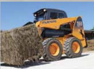
**FAST SERVICE** ▲ is achieved with the tilt-back ROPS and large engine cover that exposes internal components quickly for easy maintenance.
