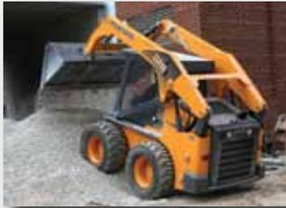
**VERTICAL-LIFT ▲** design delivers extended reach and 131-inch lift height, higher than any competitor in its weight class.
