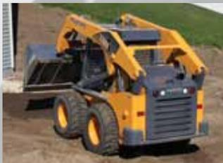
**WIDE-VIEW ▲** domed glass door option reduces glare and provides optimal visibility to the lift arm, attachment and front work area.
