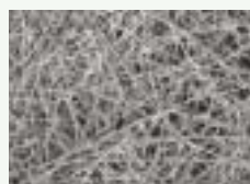
Super fine filter (glass fiber)
