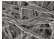
Conventional filter (paper fiber)
