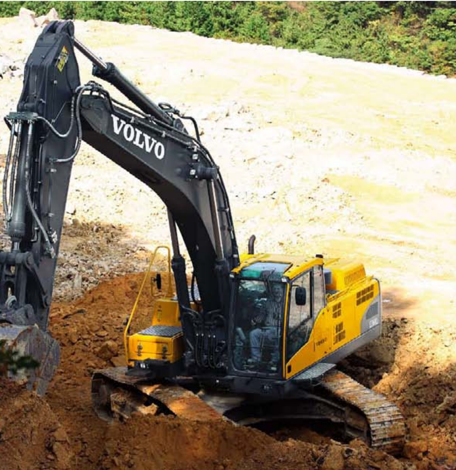
• Lifetime greased sealed track link.
