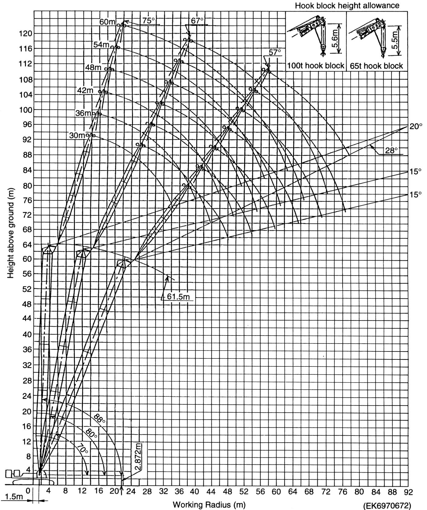
**Note:** The above working range is just under max. tower boom and jib combination i.e. 61.5m tower boom plus 60.0m tower jib.
