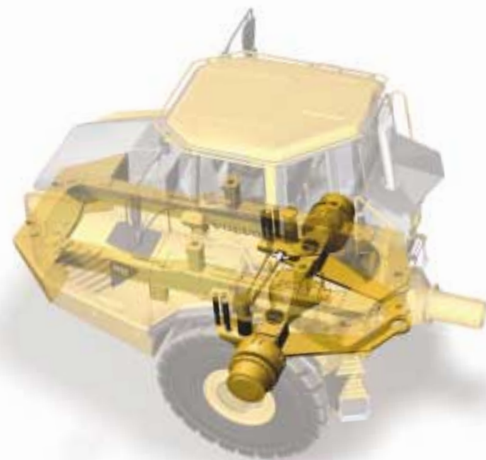
The reliable three-point suspension consists of heavy duty components. A simple and durable design that gives a comfortable smooth ride.
