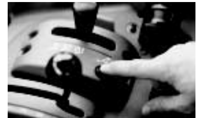
Load & Dump brake is activated with a single press of a button.
