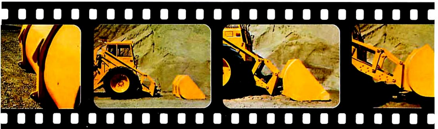
The 641 features excellent off-road negotiability and tractive power, even in difficult terrain and poor ground conditions, thanks to its large wheels, differential lock and 4-wheel drive.
