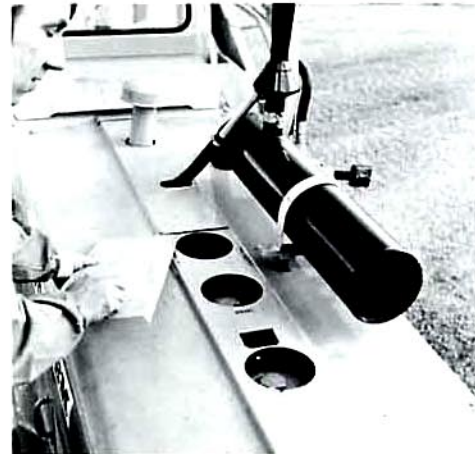
The filler points for coolant, diesel oil and hydraulic oil are assembled under one cover. An enclosed magnetic filter is also fitted in the cap on the hydraulic reservoir.
