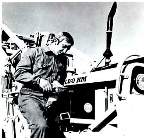
The battery can be withdrawn for inspection and topping-up by a single easy manipulation. The hydraulic reservoir is equipped with a level tube which provides instant, accurate information on the quantity of hydraulic oil.
