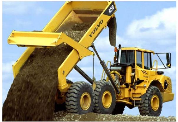
Before ordering, the material density must be quoted by the dealer to ensure the overhung tailgate and increased body capacity matched to the weight of the material will not exceed the rated payload of the hauler.
