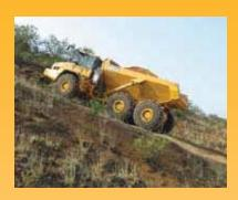
• The incorporation of a Pitch and Roll sensor in the vehicle allows the bin to not be operated if the truck is in an unsafe position.
