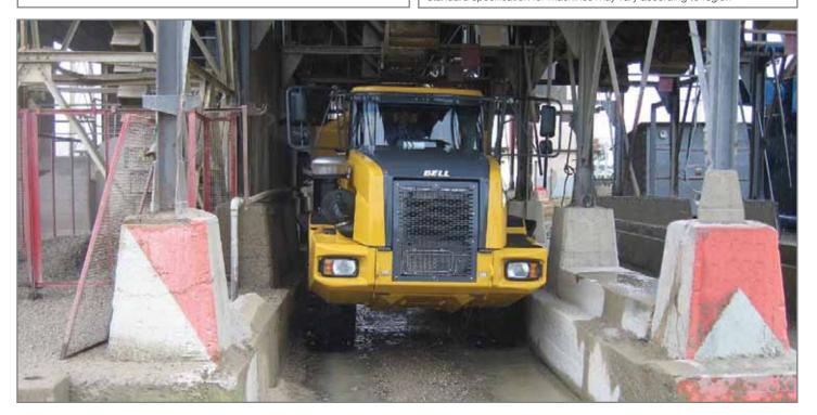
• The exclusive onboard weighing option presents the operator with real time information on the payload while the machine is being loaded. A 'limp home' mode can also be activated if the machine is significantly over-loaded.
