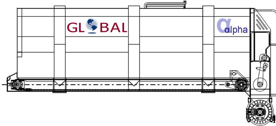
**To be mounted on existing truck- or dumper chassis equipped with power take-off, operating at engine speed, with a 400 Nm torque**
