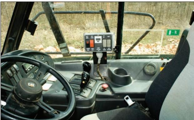
The 7460 Ejector Trailer is easy to operate. A dual-mode (Manual and Automatic), in-cab controller is used to control the trailer's apron and ejector functions.
