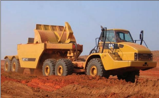
The 7460 Ejector Trailer unloads quickly, due in part to the 1281 mm (78 in) apron opening. The positive bulldozer ejector extends 102 mm (4 in) beyond the front edge of the trailer floor to minimize carryback.
