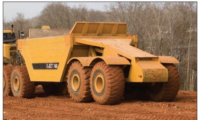
The innovative walking-beam axles allow the tires to oscillate, providing outstanding operator comfort and less haul road pumping.
