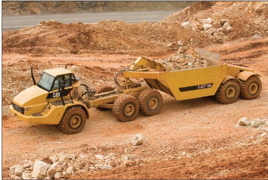
The E-Ject™ Systems 7460 Ejector Trailer expands the capacity of the Cat® 740 Articulated Truck by 40% — move more dirt faster with fewer operators and machines.
