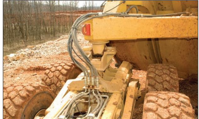
The 7460 Ejector Trailer connects to Cat 740 Articulated Trucks using a 89 mm (3.5 in) diameter pin in a fifth-wheel style hitch installed in place of the truck body and hoist mechanisms. The hitch position is centered between the truck's rear axles for optimal weight distribution when loaded.
