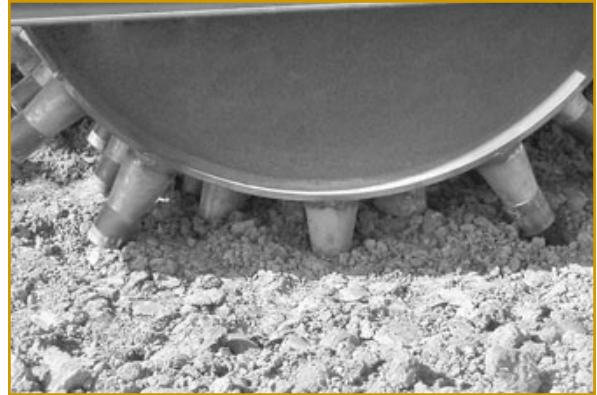
Tip surface is 7 square inches for maximum surface pressure
