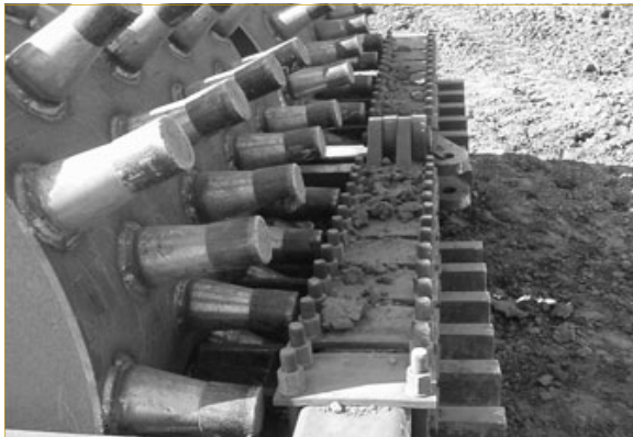
Adjustable cleaners made of a high wear resistant steel.
