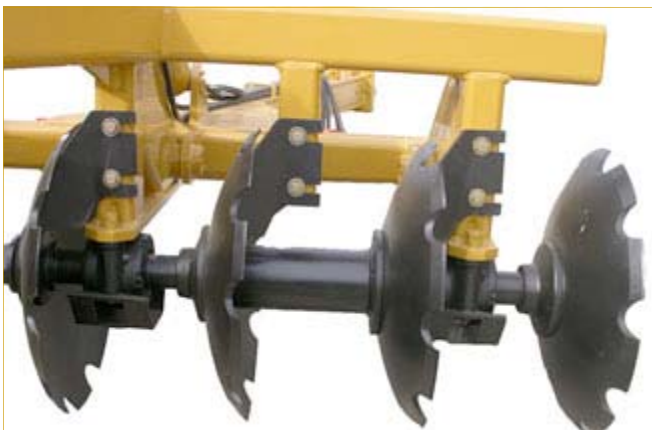
RIGID FRAME—Rails are 6" x 6" Tubing Gussets are 4" x 12" Tubing
