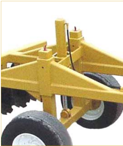
Hydraulic Lift Assembly: Tube in tube with Nylon slide bars & gusseted steel rollers. Travel position is pin locked
