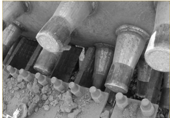
Hollow center tips allow dirt to dirt wear surface.
