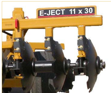
Heavy Duty Gang Supports are 4" x 6" Tubing
