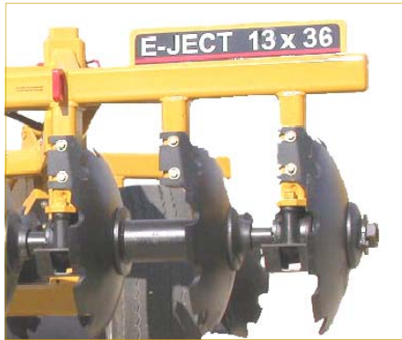
Heavy Duty Gang Supports are 4" x 6" Tubing
