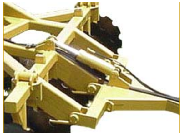
Hydraulic Tongue Adjustment is operator controlled from the cab. Adjust down force on the go. Tongue Pivot Points are 2" Dia.
