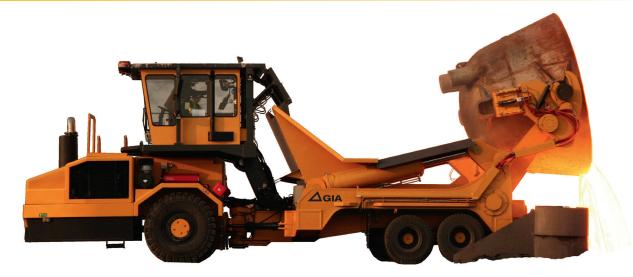
SLV 100 is a special vehicle designed to transport and dump molten slag. It is intended to be used on smooth roadways without greater slopes.
