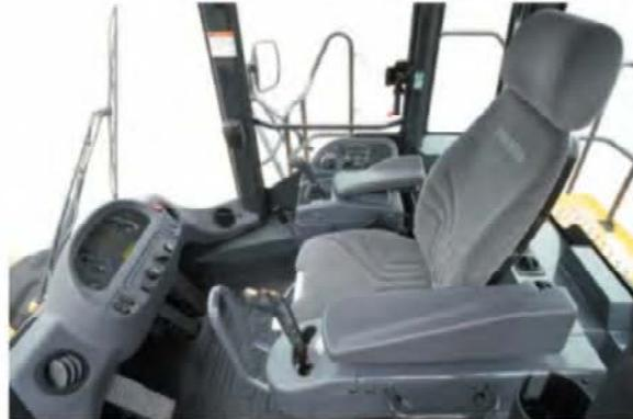
Noise at operator's ear noise level : 76 dB(A)
