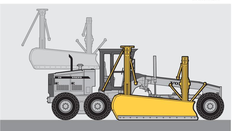
The Front Mounted Snow Wing can be used in conjunction with a snow plow as the primary plowing tool. As material is displaced from the snow plow, the snow wing is designed to displace the material far back from the road surface to eliminate snow buildup and facilitate continued snow displacement.
