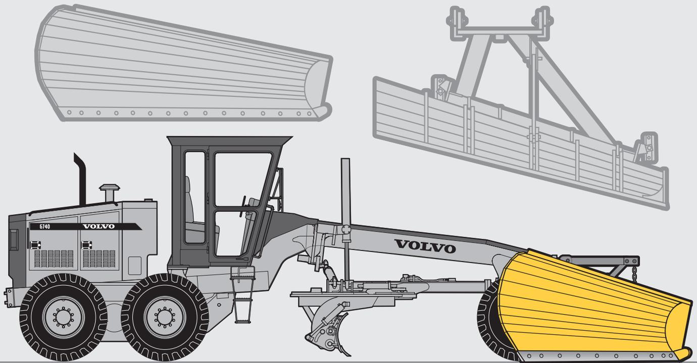
The One Way Snow Plow is used in applications where right side snow discharge only is required. Equipped with manual tip control the One Way Snow Plow “attack angle” can be adjusted for maximum clearing and efficient snow pick-up and discharge.
