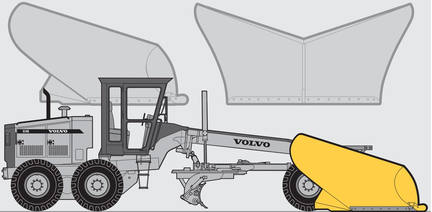
The Volvo “V” Snow Plow is designed for severe snow clearing applications such as opening uncleared roads. The “V” plow slices the material and displaces the snow in both directions for maximum single pass snow clearance at high speed.
