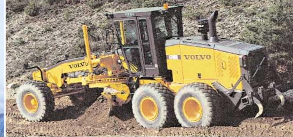
No matter how you use your motor grader, stresses constantly change, creating spike loads on the frame and front axle well in excess of the total machine weight. To keep these loads under control, the frame and axle have to take all these stresses without deflecting or deteriorating. These stresses can be further increased when the grader articulates for maximum reach or to cut ditches.
