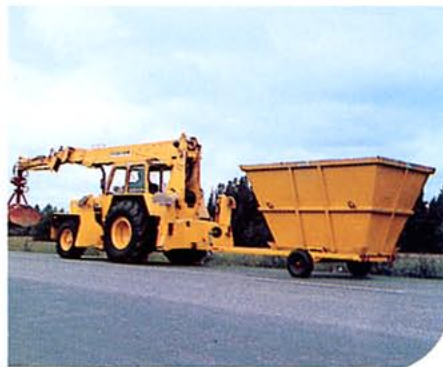
The Volvo BM 693 – a compact, manoeuvrable, highly versatile, mobile crane, with a wide range of attachments for use in modern materials handling.
