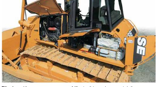
Tilt cab provides easy access Should your 1650K or 1850K need repair, the operator platform can be tilted in less than 10 minutes to provide convenient access to the for minimized downtime.
