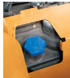
DEF tank fill
