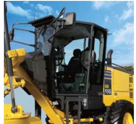
ROPS (Roll-Over Protective Structure) Cab (Equipped with defroster and intermittent wiper)
