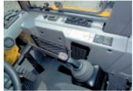
Easy, intuitive handling; nearly all operating functions are integrated in one joystick
