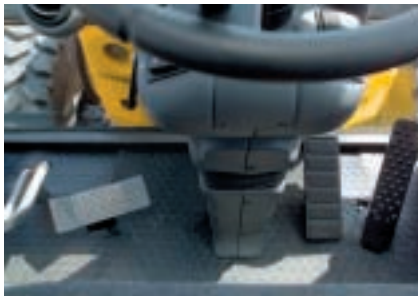
Left foot operated swing pedal avoids tiredness
